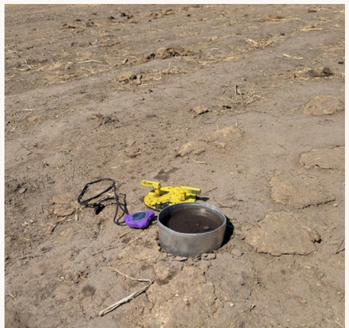
Figure 2. The crop residue from this tilled field was grazed, leaving very little soil armor. Infiltration was 0.01 inches/minute.
