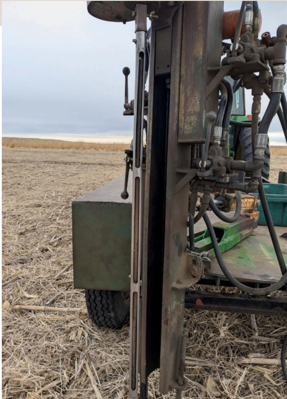
A Giddings probe was used to collect soil samples to 48” deep at Dakota Lakes Research Farm.
