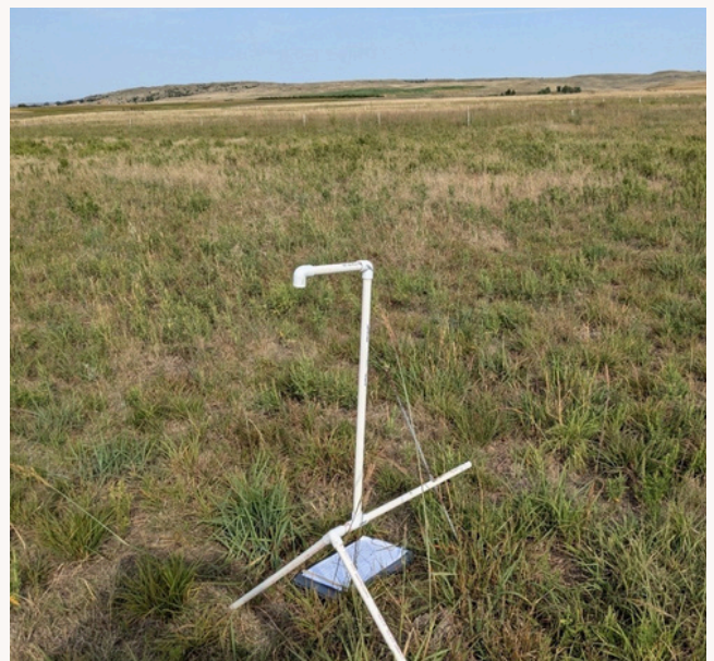
Figure 8. The tool used to collect step-point-count data. Photo taken Sep. 29 in the Shields pasture.
