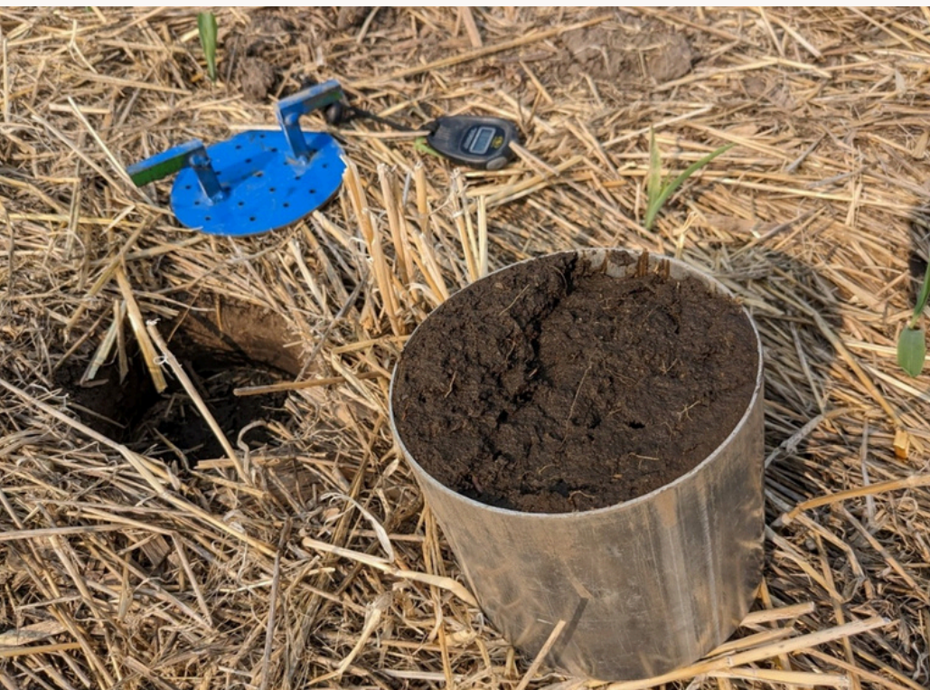
May 23, 2023. The underside of an infiltration ring. The soil is evenly wet and multiple nightcrawler channels are visible at 3" below the soil surface.
